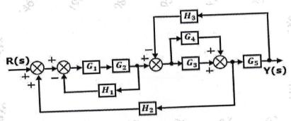
b) Obtain transfer function Y(s) / R(S) of following system using Mason's gain formula
