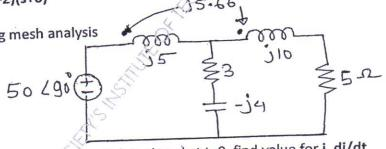
For the shown network ,switch is closed at t=0. find value for i, di/dt
