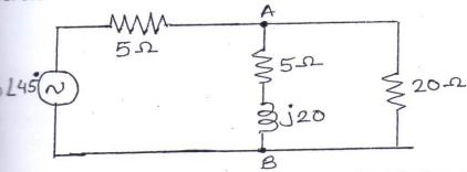
Determine Y parameters for the shown network. Also write Z-parameters from Y-parameters
