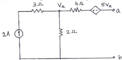
b) Find Z and h-parameters for the network shown in following figure
