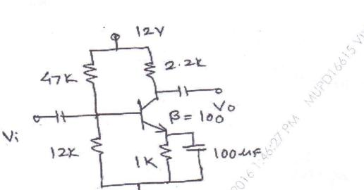
(b) Determine  $A_v$ ,  $Z_i$  and  $Z_o$  for the following circuit.
