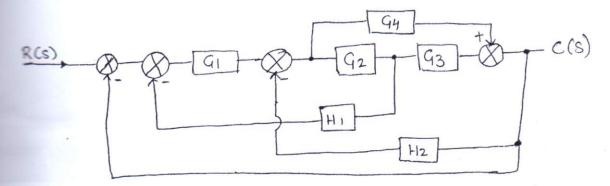
(b) For a system show determine type of the system, error coefficients and the error for the following inputs.
