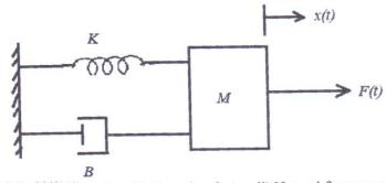
Find i) Transfer function, ii) Damping factor, ii) Natural frequency, iii) Percent overshoot, iv) Peak time, Assume: K = 33N/m, B = 15 N-s/m, M = 35kg
