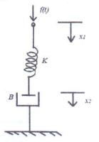
(c) Find the transfer function of the network shown in following Figure using Mason's gain formula.
