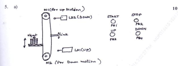
The Elevator shown in figure above employs a platform to move objects up and down. The obejctive is when UP Button (PB3) is pushed, the platforms carries object to the up position upto LSI (Link on other Side of object touches LSI) Similarly when Down button (PB4) is pushed, the platform carries object down till LS2. M1 and M2 are separate motors used for this operation Process should start only when START Button is pressed and should stop when STOP Button is pressed.
