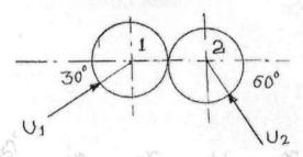
b)Two identical rollers of mass 50 Kg are supported as shown in fig. To maintain the equilibrium, determine support reactions. [6]
